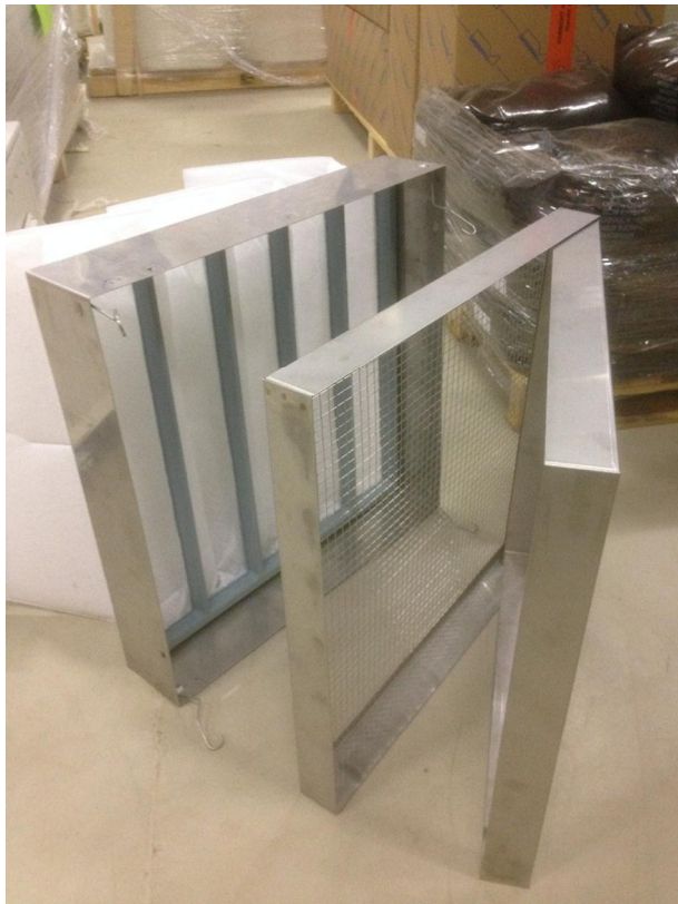
Menardi FF-B customized for prefilter, Menardi MRF, in Menardi FF-SB frame together with Winair bag filter. Filter service from inlet side (dirty side). Material AISI 3016L
