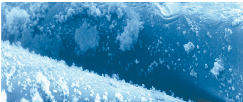
SEM image precoated individual fibers
